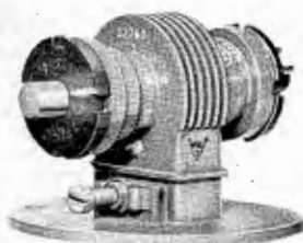
(A) Cooled by forced air flow past fins.
